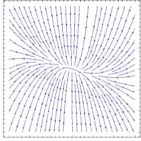
3. Does the planar system whose phase plane is shown below have two real eigenvalues, or two complex eigenvalues? What are the signs on the real portions of the eigenvalues?
