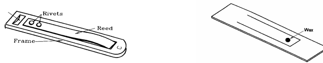
Figure 1: A free reed from an American reed organ (left) and a sheng reed (right) from Gellerman [2].
