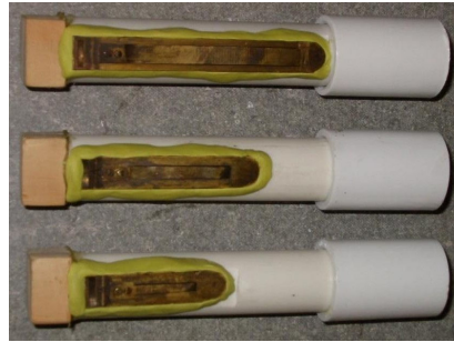
Figure 2: Free reeds mounted in PVC pipe.
